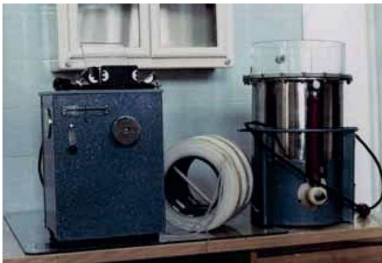
Coil kidney of Hradec Králové type. From left side: finger pump, coil dialyzer of the Chiradis type; recirculation reservoir for coil dialyzer with a pump to recirculate the dialysate.
